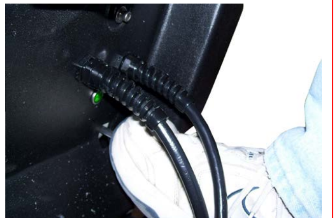
PRESSING THE PUMP PRIMING VALVE
