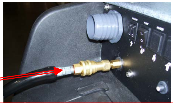
Connect the male end of the HP Solution Hose Assembly to the female solution outlet fitting on the machine. Connect the female end to the cleaning tool.
