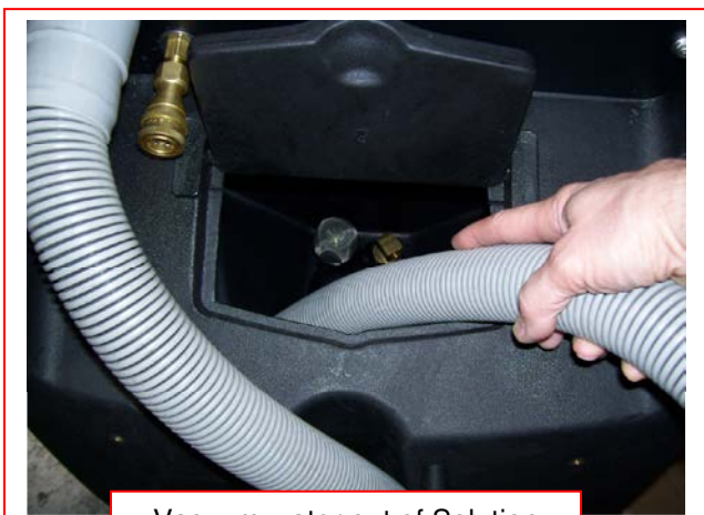
Vacuum water out of Solution Tank
