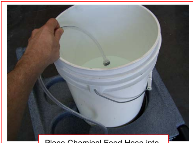
Place Chemical Feed Hose into Rinse Solution
