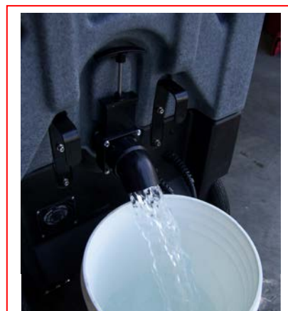
Drain water from Recovery Tank
